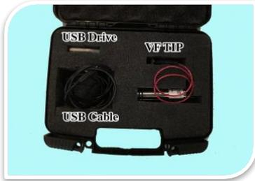
This is metal tip that is used for calibration verification. It has two set calibration standards points with the tolerances and values printed on the tip. It has one switch to transfer between the two set points. One low value and one high value allows you to linearly verify the calibration of the instrument. Comes with a case, USB Drive with software, and a USB Cable.
