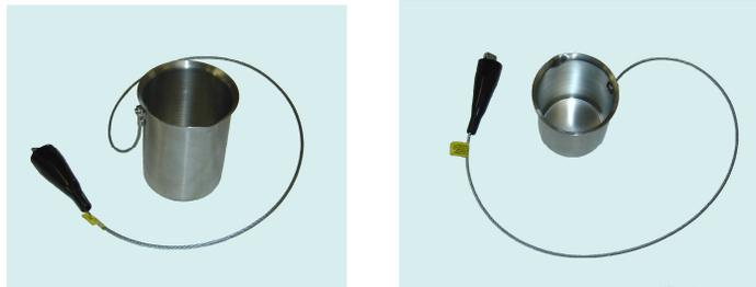
The JF-1A-HH-BK is a metal sample beaker for use with the JF-1A-HH. The metal beaker is welded with metal grounding strap to allow any DC Charges to dissipate. However, a DC Charge in the fuel does not affect the measurement of our handheld as we use AC measurement technology. The Beaker's volume is 600 mL and is constructed out of stainless steel.
