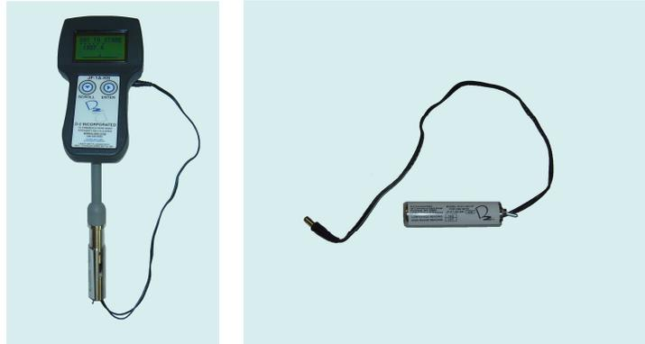
The JF-1A-HH-VF is an instrument verification fixture. This is a stainless steel device that plugs into the handheld. The tip will output two standard values, the low value is at 1% of scale and the high value is at 70% of scale. This device fits easily onto the tip of the handheld and has one switch to easily switch the range from the high to low value. This allows the user to check the conductivity calibration of the JF-1A-HH in the field with ease.
