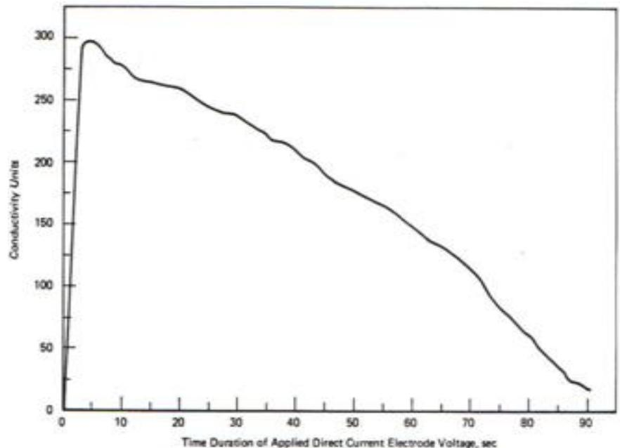
Figure 1. Polarization Effect (Typical - For Illustration Only)
